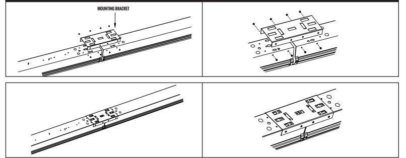
STEP 1: Screw the bracket to the end of the luminaires.
