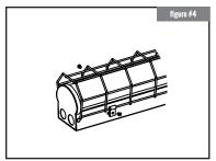
STEP 1: After installing the luminaire, Insert the provided clips(4pcs) onto the wire guard (fig. 3). STEP 2: Fasten the clips by drilling screws into the prepunched holes of fixture body (fig. 4).
