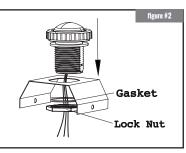
1. Knock away the knock-out hole of the end-cap. Screw the provided sensor box onto the end of housing. 2. Screw the sensor onto the sensor box cover.
